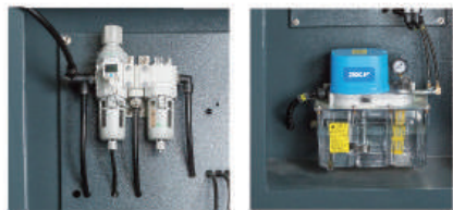
油、气系统一体式布局 Integrated Layout of Oil and Gas Systems
